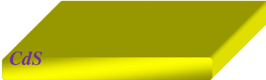
**Normally, good CdS films are obtained also by CSS. However, due to the small thickness of the CdS layer (80 nm) is preferred to use sputtering since it allows a better thickness control.**
